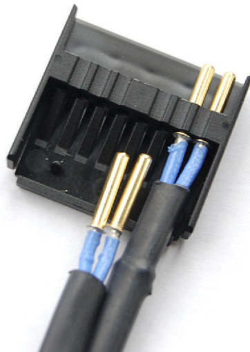
Figure 49: Inserting additional probe wires
